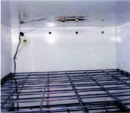
The sensor for the greenhouse controller is mounted to the ceiling inside the kiln. The four holes drilled through the upper back wall of the freezer can be seen.
