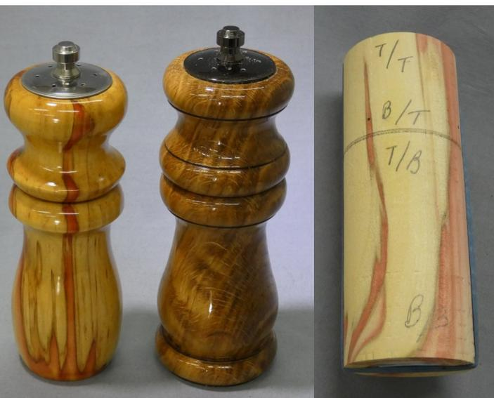
Charles Jennings made a great presentation on how to make combo salt/pepper mills especially if making them in any quantity using a homemade mandrel. He showed how to mark sections to keep them in order when turning.
