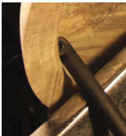
Fig 2. Undercutting the rim with the 3/8" Hunter Carbide Tool.
