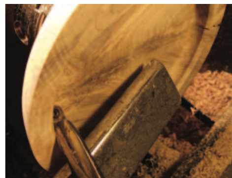
Fig 1. Undercutting the rim with the 1/2" Hunter Carbide Tool
