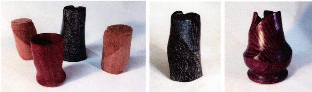
Examples of Twisted Turnings Using the 3-Point Off-Axis Method
