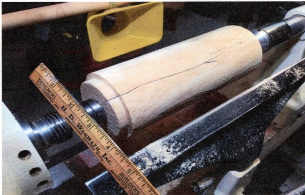
Turned 3-inch Cylinder with 2 ½ inch Diameter End Tenons
