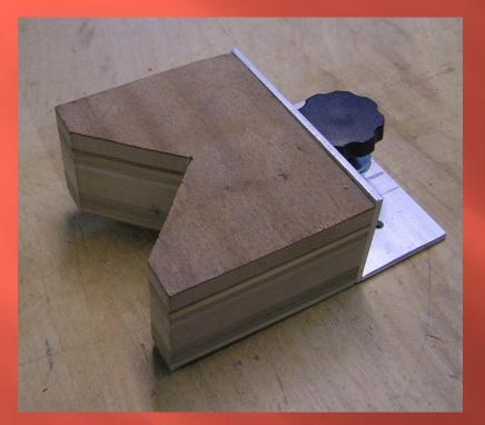
2" Aluminum Angle 4 <sup>1</sup>/<sub>2</sub>" to fit V Block
