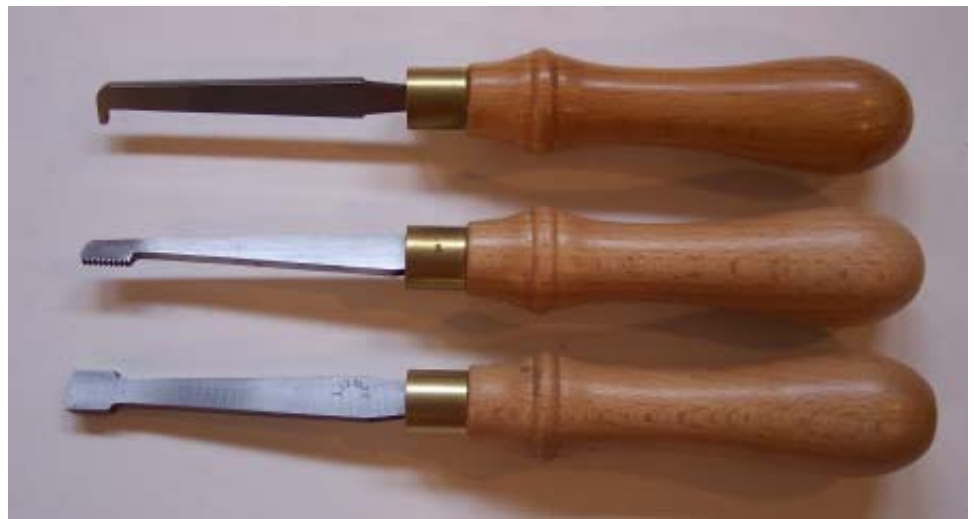
This set of Ray Iles thread chasers are the best that I've used. Bottom is outside chaser, middle is inside chaser, and top is recess cutter for inside threads.
