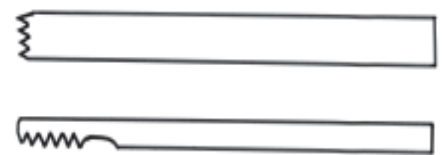
Fig. 1. Chasers have a cutting section that is very similar to an inside section of a threading die. They are made by pressing the cutting section of the chaser against a rotating mandrel that is similar to a large tap of the given thread and pitch. The outside chaser (top) has the cutting section on the end of the tool and the inside chaser (bottom) has the cutting section on the side of the end of the tool. Normal wooden handles are generally added to these tools.
