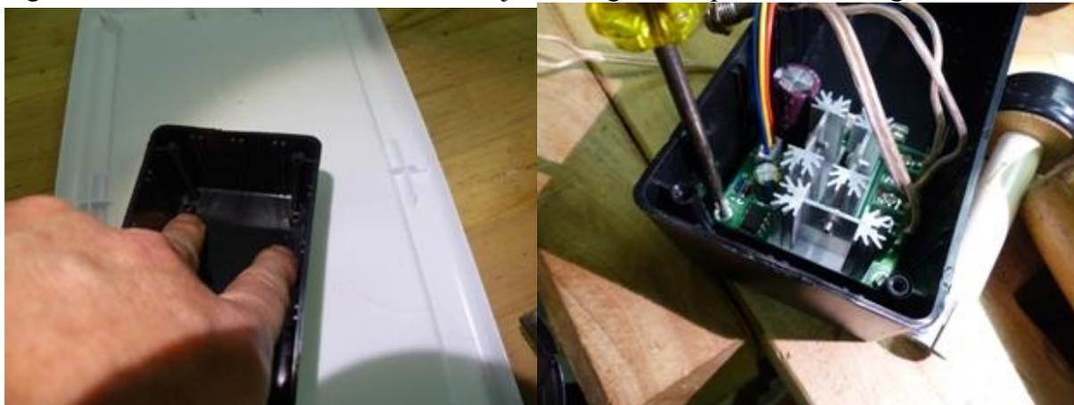
At this point you can drill 2 holes through the bottom of the box and mount it to your plywood base.
