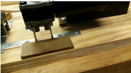
I have found it works better to place hardboard pad for the motors transmission to rest on because the motor is a little larger than the transmission.
