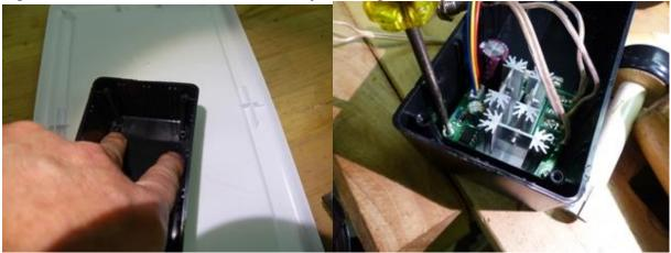
At this point you can drill 2 holes through the bottom of the box and mount it to your plywood base.
