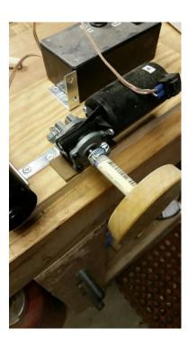
Because the motors lugs are mounted to the L brackets, it can be rotated up so maybe you could use it as a turntable for spraying......It's only an option and costs only another L bracket (see above) for a stop.
