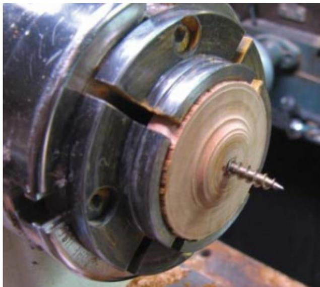
Homemade screw chuck to hold the blank for turning.
