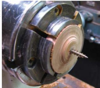
Homemade screw chuck to hold the blank for turning.
