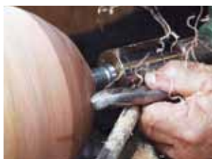
A light touch and a sharp edge will produce fine shavings and a cleanly cut surface on the outside of a bowl.
