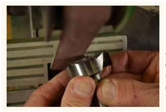
Then I sharpen the top edge of this bevel. You have to be careful when grinding this edge. You have to stay away from the center and avoid touching one of the teeth on the outside rim. It's also important to grind the relief angle. I set the bit on the sanding belt with the machine turned off. This lets me find
