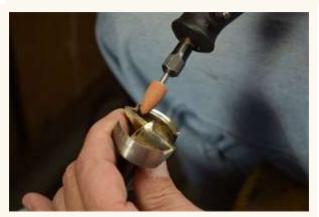
If you have bits that have a smooth outer rim use the Dremel and abrasive stone. I use one of the cone shaped ones but I've tried lots of different ones and they all seem to work. The last thing to do is to get rid of the burr's left on the outside. I use a diamond hone to remove the burr from the outside. Just lay it flat on the outside bevel and rub until it's smooth.
