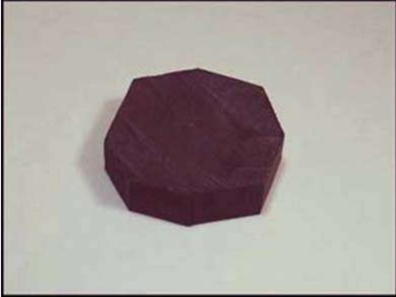
Cut a blank, larger than the hole, to turn for the collar. I prefer to make the collar out of a contrasting wood.
