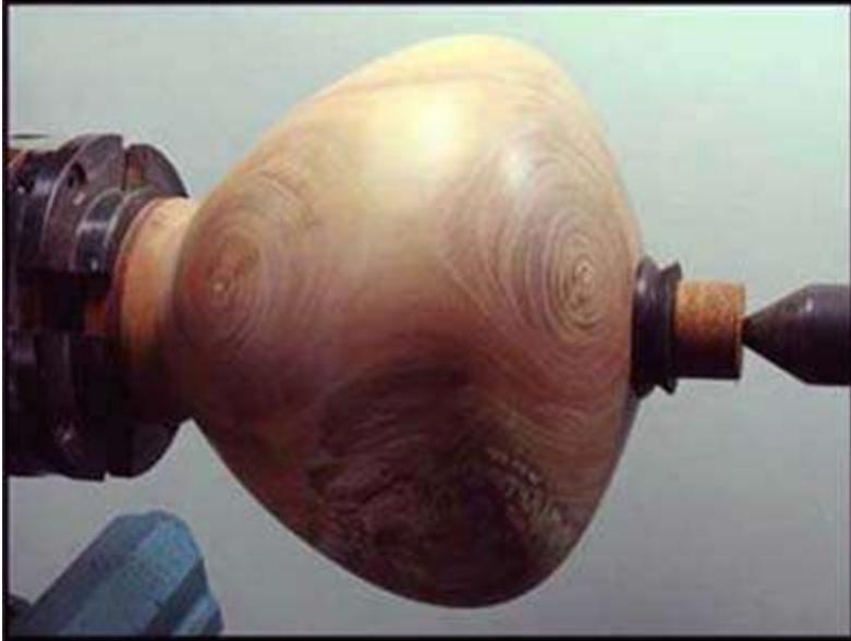
Remount the hollow form and glue in the collar. Use the tail stock to hold the piece until the glue dries. Do not put too much pressure on piece.
