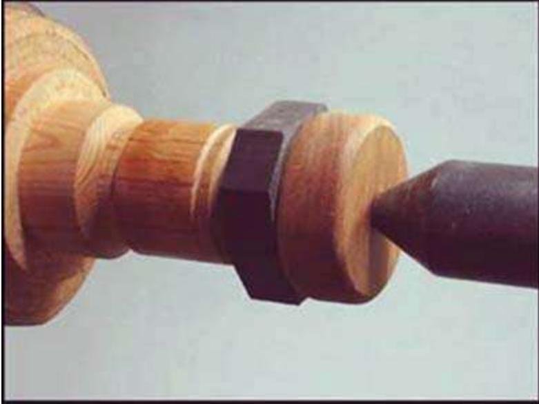
Use another waste block and bring the tail stock up to put pressure on the collar blank. Tighten the tail stock and keep the tension on for a few minutes to allow the collar blank to stick to the double sided tape.
