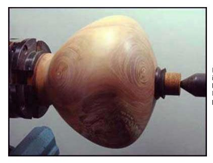
Remount the hollow form and glue in the collar. Use the tail stock to hold the piece until the glue dries. Do not put too much pressure on piece.
