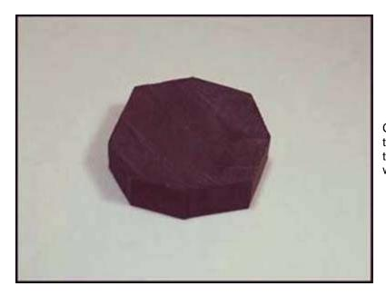
Cut a blank, larger than the hole, to turn for the collar. I prefer to make the collar out of a contrasting wood.
