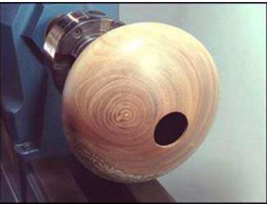
Carefully measure the diameter of the hole in the hollow form.
