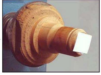
Use a waste block to mount the collar blank on the lathe. I use double face tape to attached the collar blank to the waste block. Use a waste block smaller than the collar blank so you can turn and sand the top edge.
