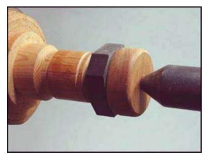
Use another waste block and bring the tail stock up to put pressure on the collar blank. Tighten the tail stock and keep the tension on for a few minutes to allow the collar blank to stick to the double sided tape.
