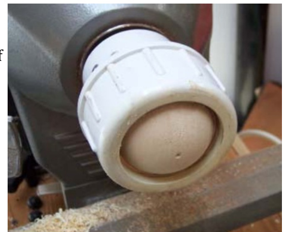
Photo 2. Ball held in ball chuck with center marked
