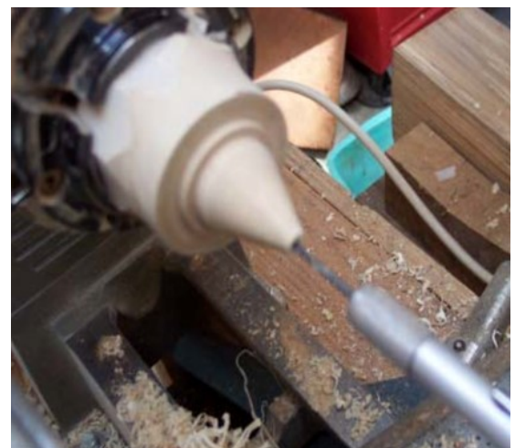
Photo 7. Drilling the 3/32" hole in the cone
