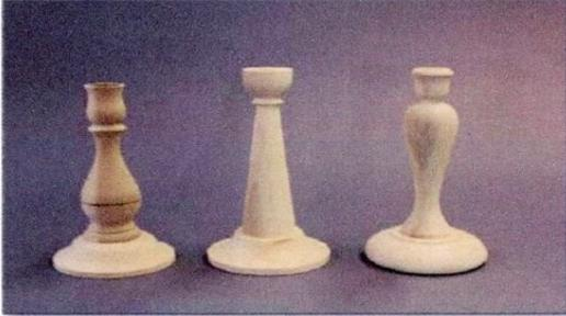
This project has two components, the base turned on a chuck and the spindle or post turned between centers. It's a great gift for mom. The project will utilize both faceplate and spindle techniques. You will use a 3/8" bowl gouge to make the base and a spindle roughing gouge and spindle gouge to make the spindle.
