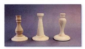
This project has two components, the base turned on a chuck and the spindle or post turned between centers. It's a great gift for mom. The project will utilize both faceplate and spindle techniques. You will use a 3/8" bowl gouge to make the base and a spindle roughing gouge and spindle gouge to make the spindle.
