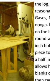
the log. He finds blades very reasonably priced at Holston Gases, 1105 Stuart St, Chattanooga. His homemade jig fits on the bandsaw and he mounts round wooden plates with a ½ inch hole to the bottom of the piece to be cut. The plate fits in a half inch movable peg which allows him to cut out bowl blanks of various sizes. These then can be mounted on the
