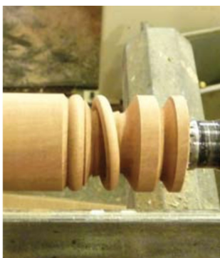
Figure 5. Starting the second loose ring.
