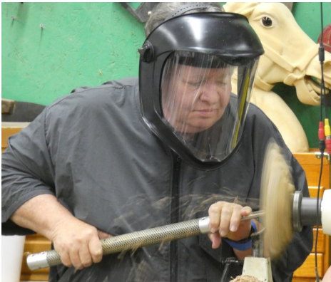
Peg Schmid mounted a burl with a faceplate on the backside
