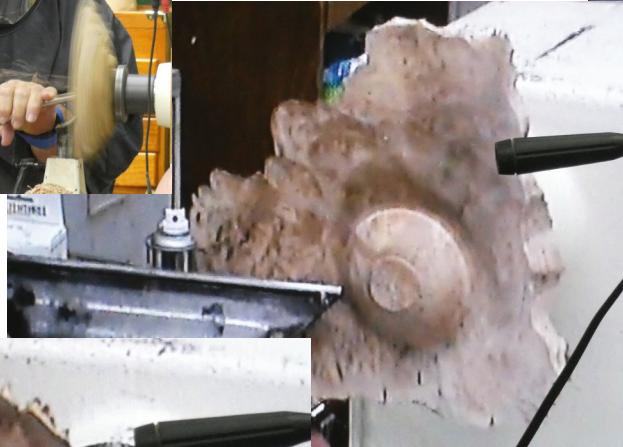
The bowl was turned and hollowed out. A finial made to fit the hole. Then the holes
