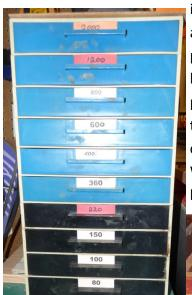
into quarters and returned to the drawer. A quarter sheet is folded into thirds and put in a tray in front of the lathe. When worn-out it's thrown away and replaced in the tray. The pneumatic sander is hung on the shelf in front of the lathe. Roloc foam disc holders, hook & loop 2" sanding discs (60-3000 grit) in a plastic box are stored next to the lathe in the drawer of a rolling tool box. An ex-
