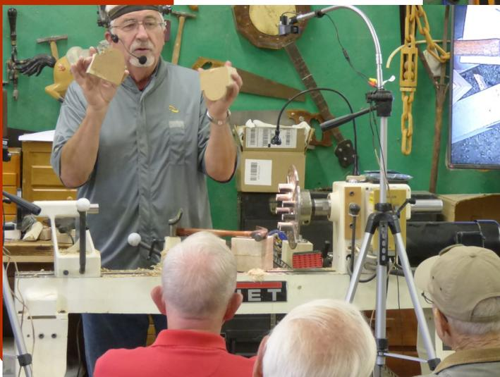
Mounting the bowl for turning in the Cole Jaws
