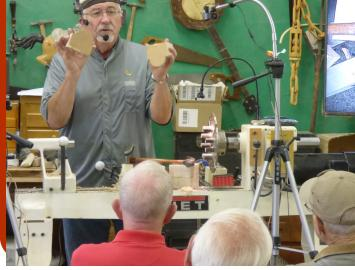
Mounting the bowl for turning in the Cole Jaws
