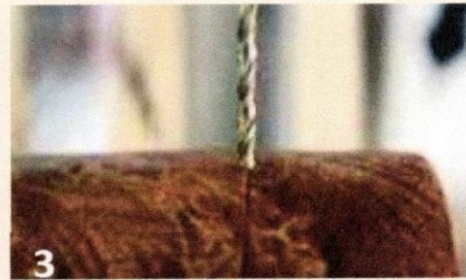
Tape the lid to the box securely before drilling. Use a shopmade V-block to hold the round box and then drill a pinhole centered on the box/lid juncture.
