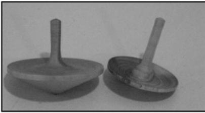
Here are a couple of my tops. The one on the left was made from a solid chunk of wood while the one on the right is made from a fabricated top blank using a slice of an oak tree branch and a maple dowel. Note the cupped or bowl-shaped top part of the main body. I've found that tops turned like this spin better than flat or domed tops.
