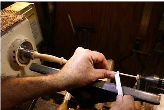
I might support the right end by crossing my hand over the tool. I have had some very thin shafts vibrate regardless of what I did. I don't worry about it too much when shaping but it's horrible when doing the finish cuts. Instead of resorting to sandpaper, I use a small cabinet scraper.
