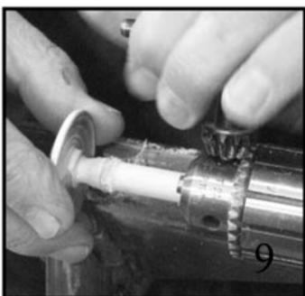
Sand the bottom of the top while supporting with a finger of the left hand. At this point the stem is very fragile. Sand the top of the top body while supporting it with the fingers of the right hand. Fold the sandpaper until it is narrow enough to properly sand the stem of the top. Do not exert too much
