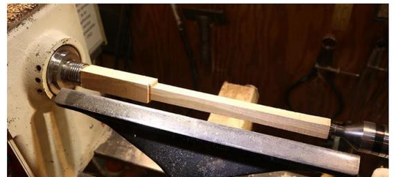
**Tools:** Skew chisel, small roughing gouge, spindle gouge for handle detail. A spindle gouge can be a problem on the thin shaft since a small vibration can make the wood ride up over the tip and cause a catch. A skew is better since the flat bevel supports the edge. A small roughing gouge would be my second choice, acts a bit like a curved skew. Tools should be very sharp. I usually hone and strop on leather.
