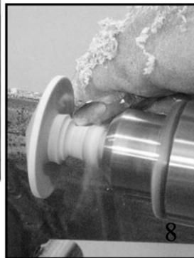
It is important to leave a little step up from the lowest point of the dish to provide additional support of the glue joint. See photo of the finished top.
