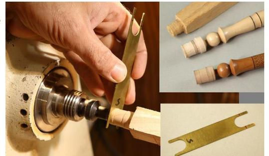
**Getting ready to turn:** For this exercise I picked a Black Cherry blank from my stash of wand blanks. These two photos show the blank, first with the Morse taper cut, then with it jammed into the lathe spindle. Bring up the tailstock to seat it firmly then release
