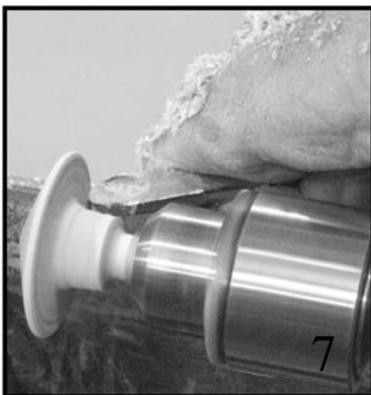
I like to hollow the top side of the top body to give it a dished form. I find tops turned this way spin better and longer. As the dishing is started, as much material as possible is left near the center.
