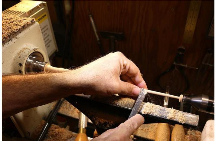
the tip and support the end of the handle by forcing it against the underside of my forearm. This supports the tool well. Note that as the tool is moved along the shaft, the left hand has to move with it. The pressure needed for support is very light if the cut is very light. As Richard Raffan said, if the wood gets hot from friction on your hand, you are using too much force with the tool!
