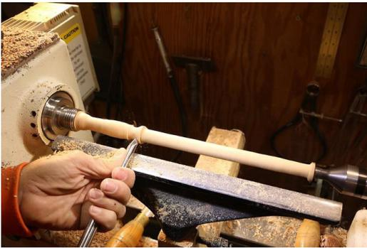
Begin tapering and shaping the shaft. I generally use a skew chisel for this. A small roughing gouge will also work. As the shaft gets thinner the fun begins. When it starts to get thin the shaft will probably start to vibrate and chatter during the cut or it may even vibrate on its own without even touching it.
