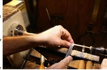
the tip and support the end of the handle by forcing it against the underside of my forearm. This supports the tool well. Note that as the tool is moved along the shaft, the left hand has to move with it. The pressure needed for support is very light if the cut is very light. As Richard Raffan said, if the wood gets hot from friction on your hand, you are using too much force with the tool!
