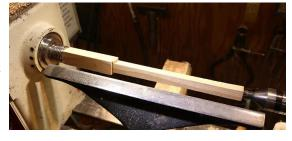
**Tools:** Skew chisel, small roughing gouge, spindle gouge for handle detail. A spindle gouge can be a problem on the thin shaft since a small vibration can make the wood ride up over the tip and cause a catch. A skew is better since the flat bevel supports the edge. A small roughing gouge would be my second choice, acts a bit like a curved skew. Tools should be very sharp. I usually hone and strop on leather.
