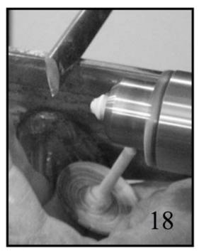
Once the waxing is done, part off the top with a skew chisel. Make a deepening "V" cut at the end of the stem. This provides a pointed stem, which allows the top to be spun upside down.
