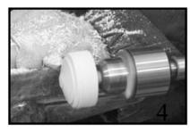
Face off the end of the top blank at a slight slope. I begin this cut with the flute straight up and then roll the flute over as the cutting begins so that the cut down the face is a nice shearing cut. Begin to form the taper of the bottom part of the top body. Continue making cuts starting at the outside rim and continuing toward the center of the spinning blank. After entry, rotate the flute to point away from the
