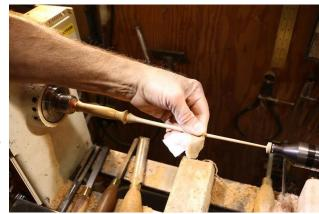
with the lathe running and melted into the surface with friction from a small piece of cloth.
