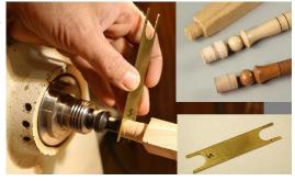
**Getting ready to turn:** For this exercise I picked a Black Cherry blank from my stash of wand blanks. These two photos show the blank, first with the Morse taper cut, then with it jammed into the lathe spindle. Bring up the tailstock to seat it firmly then release
