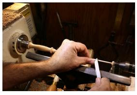
I might support the right end by crossing my hand over the tool. I have had some very thin shafts vibrate regardless of what I did. I don't worry about it too much when shaping but it's horrible when doing the finish cuts. Instead of resorting to sandpaper, I use a small cabinet scraper.
