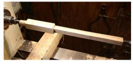
a little. Too much force on the tailstock can cause problems such as bending and splitting when the shaft gets thin. Think about the design - end, handle, transition, shaft, and tip. For small children avoid points.
