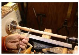
Begin tapering and shaping the shaft. I generally use a skew chisel for this. A small roughing gouge will also work. As the shaft gets thinner the fun begins. When it starts to get thin the shaft will probably start to vibrate and chatter during the cut or it may even vibrate on its own without even touching it.
