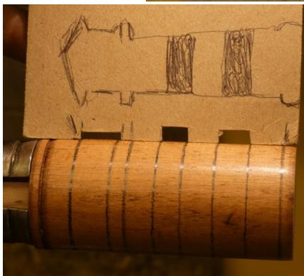
lines between each section. The whole thing from 5 to 1 could be turned and the sections marked again with the storyboard. A groove was cut with the toe of a skew then lines burned to mark out the sections. This will help keep colors from running later. (#s on storyboard)
