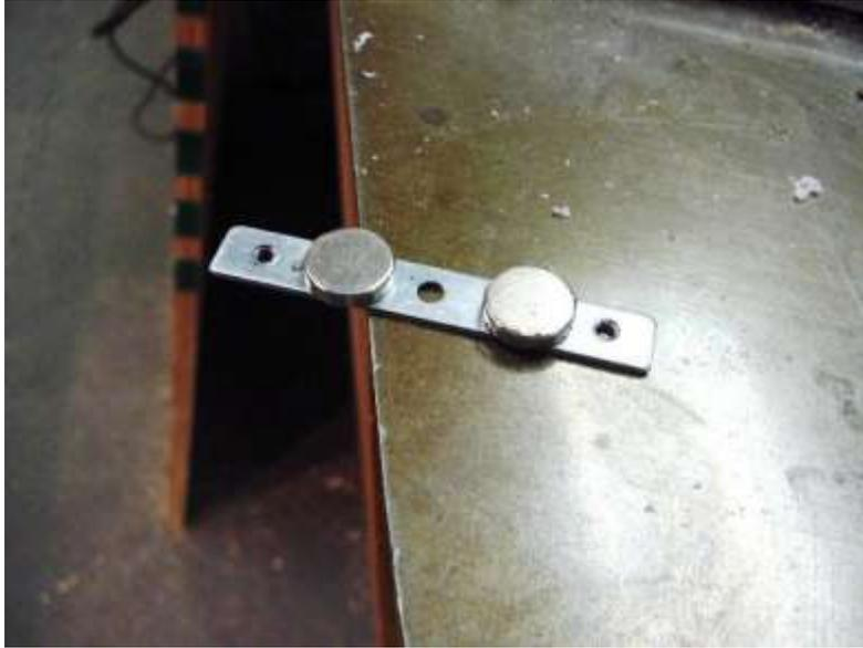
I then slip a piece of heat shrink tubing over the strip and magnets.
