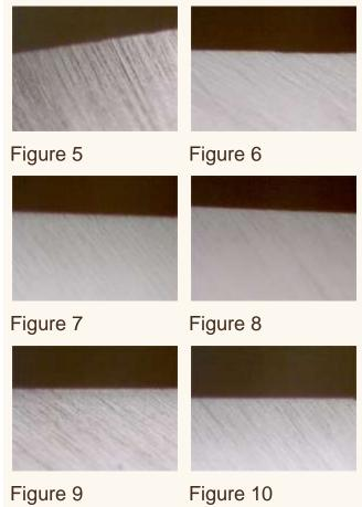
Figure 5 sharpened on a Lap-Sharp™ with 10? Trizact.
