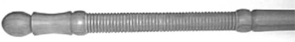
Even though these pieces were only about 29-30 inches long, I had to use a steady rest to stabilize the wood for turning. On small things like lace bobbins and treen, one can normally stabilize it with their fingers. I simply couldn't do so on something this size.
