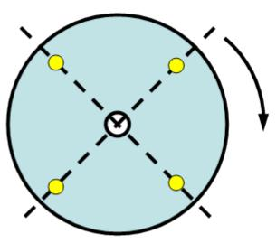
Rotate 45° after 1<sup>st</sup> four tests and repeat the test on four more spots
