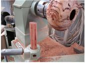
The position of the swing point of the compass and height of it, all have a bearing on the scribed arc. I use the banjo with a hardwood peg elevated in the toolrest hole. The hardwood pin, I split up quickly and have been meaning to turn up a more professional looking pin. But it does show you don't need anything fancy here.
