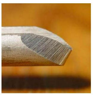
**TURNER:** Dave Peebles **TOOL:** Bowl Gouge **COMMENTS:** This is my 5/8" V-15 Glaser gouge. I use this for about 90% of my work. It has a little longer side grind than my other gouges. This is also the gouge that I do most of my shear scraping with. The nose bevel is about 62 degrees.
