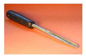
**TURNER:** David Ellsworth **TOOL:** 3/4" diamond parting tool **COMMENTS:** Here is the grind I prefer for my parting tools because of the mass and support that the curved lower bevel brings to the edge, eliminating most vibration.
