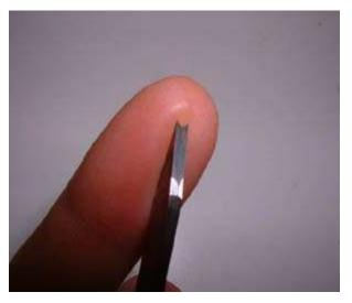
**TURNER:** Dave Peebles **TOOL:** Bowl Gouge **COMMENTS:** This is my 3/8" V-15 Glaser gouge. I use this for detailing work. It works very well for forming tenons for mounting in the chuck. I also use this gouge for making a last clean up pass on difficult woods. The nose bevel is also about 62 degrees on this one.
