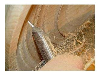
**TURNER:** Russ Fairfield **TOOL:** Continental bowl gouge **COMMENTS:** I use a Continental Spindle Gouge when I need a smooth cut on the inside of a bowl. I grind the tool with a blunt fingernail shape and usually with a 40° tool angle, but that can be changed for the task at hand.
