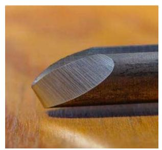
**TURNER:** Dave Peebles **TOOL:** Bowl Gouge **COMMENTS:** This is my 3/4" V-15 Glaser. I use it mostly for roughing out large blanks. It removes a lot of wood in a hurry. This is basically the way it was ground when I bought it. The nose bevel is about 65 degrees.
