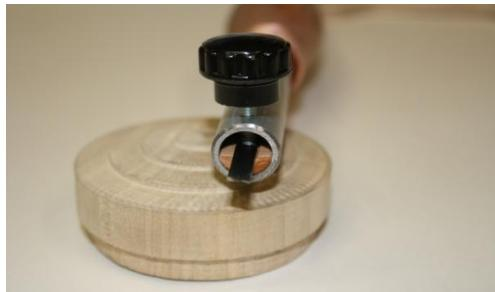
Mix some 5 minute epoxy and spread some around the inside of the hole in handle and immediately place un-cut end of pipe inside the hole until it bottoms out. Glue the half-dowel inside the pipe with the same epoxy. Place the blade immediately into the groove in dowel, screw the knob into pipe and tighten against the blade. This will help hold the dowel into place while the epoxy cures.
