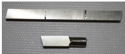
Close up view of 3/16 square HSS cutter bits. They can be purchased in  $2\frac{1}{2}$  inch lengths or 4 inch lengths. A  $2\frac{1}{2}$  inch piece can yield 3 bits that are substantial enough for use when evenly divided. They can be scored with an abrasive disc on a Dremel or other similar rotary tool and then broken apart. About 1/3 of the
