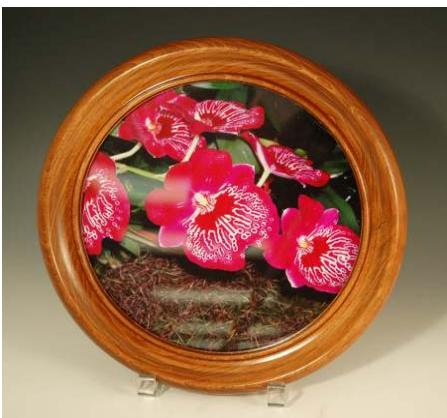
photographs, so the frames didn't have to be overly large. The dimensions I settled on were: outside diameter, 5"; inside diameter, 3 and 3/8"; thickness from back to highest point on front, 5/8". A cross-section of the frame pattern I used follows (**Figure 1**), and I'll describe how to make it, but there are many variations possible.
