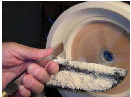
of the skew, cut two lines to define the width of the accent bead (**Figure 7**). Remove the wood between the bead and the inner opening using the
