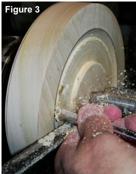
back of the frame (the front edge will eventually be removed anyway!). Next, start cutting the center opening at the back of the frame using a 3/8-inch spindle gouge (**Figure 3**). Make this opening deep enough to accept the picture, Plexiglas and picture backing (about 3/8-inch) and wide enough to accommodate the width of your scraper.
