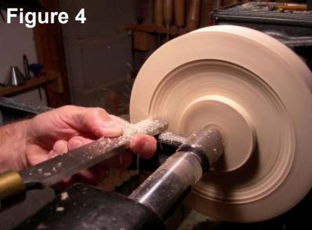
sure that the upper left corner of the scraper face is slightly above center and that the length of the tool is parallel to the ways of the lathe. When the cuts are finished, sand the back and the outside edge of the frame. (Only sand to 150-grit if the frame is to be stained – see Sanding and Finishing).
