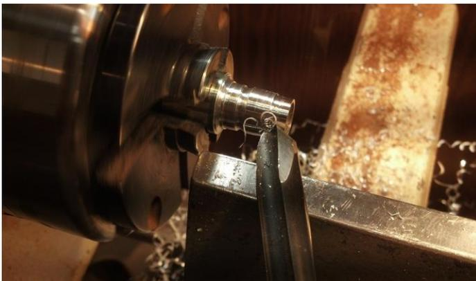
Use a spindle gouge, parting tool, skew, bedan, or scraper to turn the embedded end to the final diameter. Measure often.
