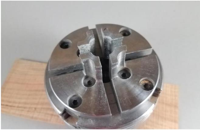
I use Nova chucks. My favorite jaws for 3/8" to 1" rod are the NOVA 6026 mini spigot jaws. The Nova pin jaws are also useful but won't quite close on a 3/8" rod. Before I got the mini spigot jaws I would wrap a few layers of aluminum tape around the.
