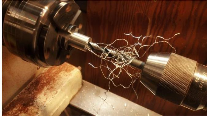
NOTE: the hole can be drilled at any point – drill the unturned blank or at any step during the turning. I usually drill into the EXPOSED end after I grip the EMBEDDED end.
