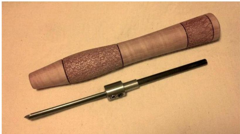
Since I have a lot of these inserts, I buy tools without handles. This not only reduces the cost but tools without handles don't take up very much storage space. I keep a couple of dozen turning tools in one shallow drawer within arm's reach of the lathe.
