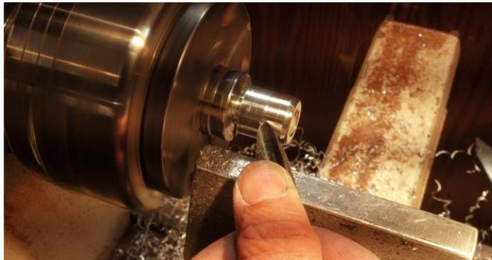
Turn what will be the exposed surface of the insert just enough to clean up the metal surface.
