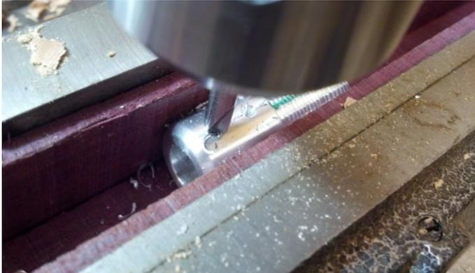
Prepare a v-block or means to hold the insert to drill the holes for the set screws. Mark the locations and use a center punch to dimple the metal for the drill bit. With the mark at the top, hold the blank securely, and start each hole with a center drill bit. I hold the part with a machinist's vise.
