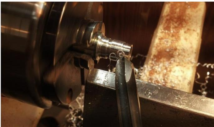
Use a spindle gouge, parting tool, skew, bedan, or scraper to turn the embedded end to the final diameter. Measure often.
