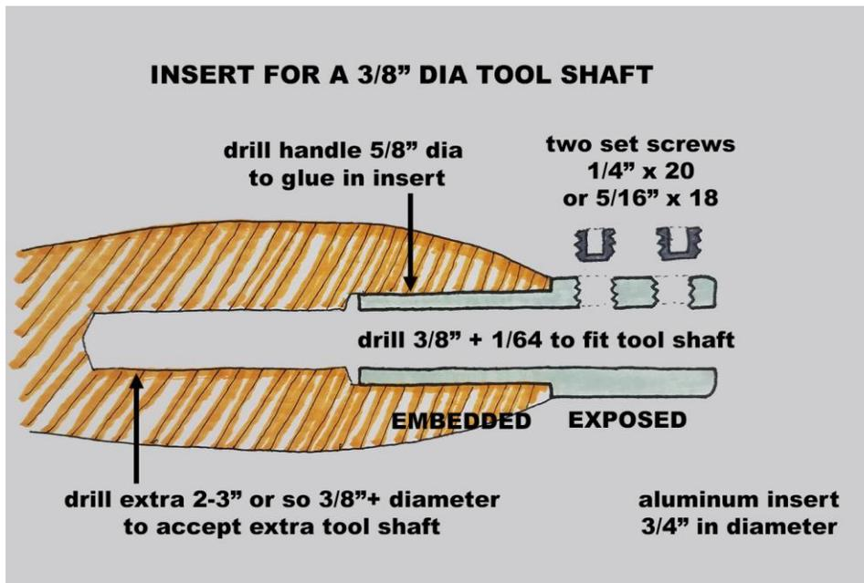
Drill a hole to fit the embedded section of the insert and a longer hole to clear the end of the tool shaft if desired. Support the handle blank with the tailstock (cone or wood end for the live center to fit the hole). I like to turn the handle so it merges nicely with the insert. Sand and perhaps
