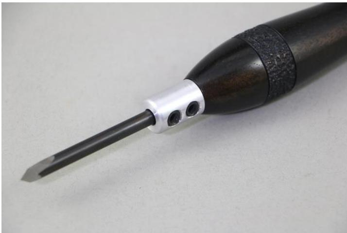
Some inserts I bought were a much larger diameter than needed, making them awkward to hold. For example an insert made to hold 1/4" diameter tools was 1" in diameter – way too big.
