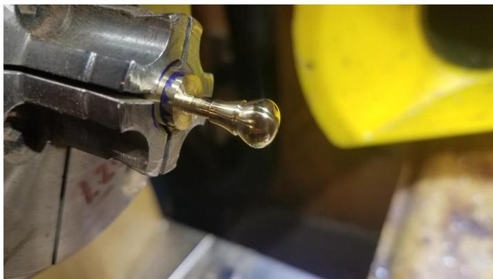
One of the three feet ready to cut off the lathe.
