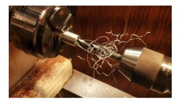
NOTE: the hole can be drilled at any point – drill the unturned blank or at any step during the turning. I usually drill into the EXPOSED end after I grip the EMBEDDED end.
