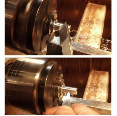
Decide on the set screw size and thread. For this size insert I usually use 1/4"x20 tpi set screws and sometimes 5/16"x18 tpi. Consult a thread chart for drill size. For example, use a #7 drill for a 1/4x20 set screw. Home Depot and others sell an inexpensive set containing a tap and the proper drill bit.
