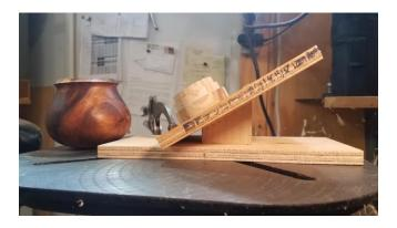
I drilled the three holes evenly spaced around the bottom of the box, 120 degrees apart
