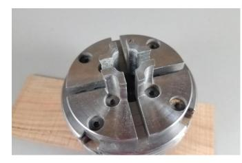
I use Nova chucks. My favorite jaws for 3/8" to 1" rod are the NOVA 6026 mini spigot jaws. The Nova pin jaws are also useful but won't quite close on a 3/8" rod. Before I got the mini spigot jaws I would wrap a few layers of aluminum tape around the.
