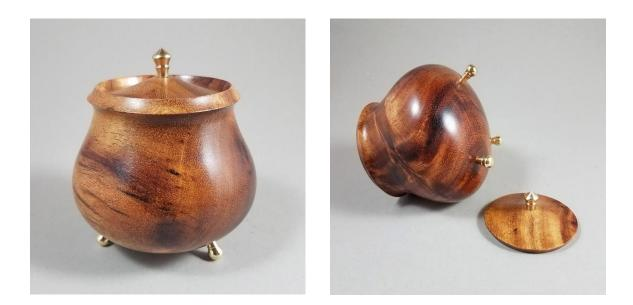
The best type of brass for turning is the 360 "free machining" alloy. It turns nicely with HSS parting tool, spindle gouge, and other tools.
