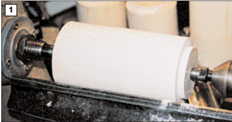
1 Rough out between centers with a 1 1/4" roughing gouge. With a 3/8" bedan tool, cut a 2" x 3/8" tenon (for fitting the blank into a scroll chuck) in one end.
