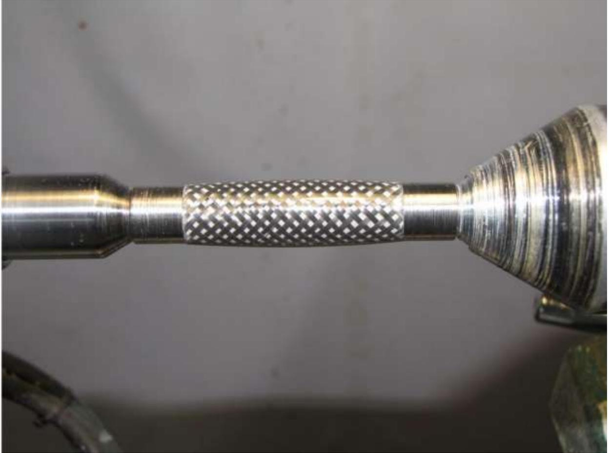
Assembled it to the rest of the WSII components and wah-lah a stainless steel Wall Street II PENCIL. Didn't have any pens and this 0.5mm pencil had been lying in a drawer for a couple years so I thought I would use it.
