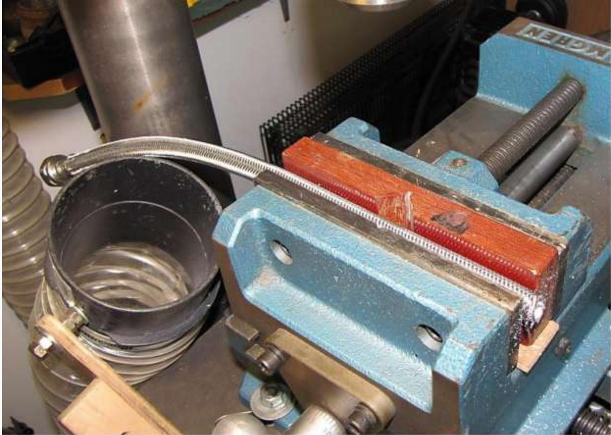
worked the braid off of the rubber, tied it with some small wire around a Wall Street II pen tube which I had painted white then cast the whole thing in clear Alumilite. Turned it between centers, applied 4 coats of CA(Alumilite doesn't shine like PR) then polished it with Micro Mesh starting with 2400 then thru 12000.
