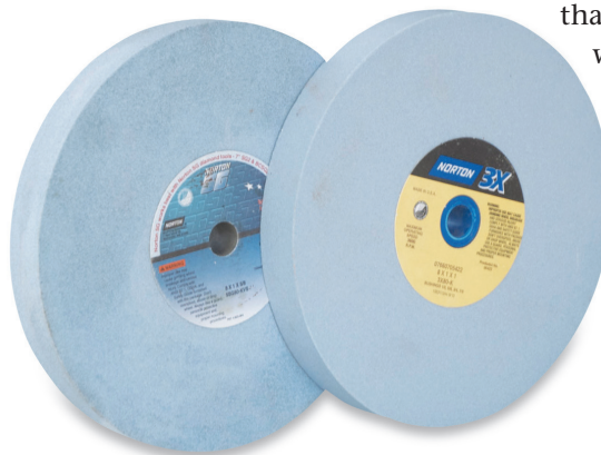
Ceramic wheels. On the left is a Norton SG wheel and on the right, the 3X wheel. Both cut faster and cooler than aluminum oxide wheels. The SG wheel lasts a very long time. In fact, the wheel on the left has been in daily use for over two years.
