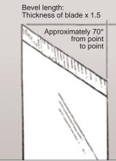
Typical grinding of a skew chisel
