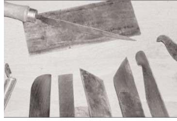
craping tools are quite similar to the cabinetmaker's scrapers shown with a burnisher). Both types of scrapers usually cut with a n make use of a burnisher to raise that burr. Turning scrapers are th in weight and come (or can be made into) in an array of shapes for poses.
