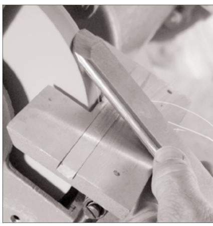
Using the back edge of the tool rest, pivot the curved skew to grind the edge. Us rotational movement, grind in the area that is roughly parallel to the face of the w
