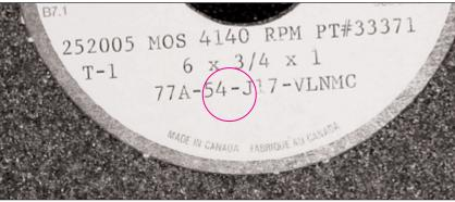
It is challenging to look at a wheel and guess its grit size and hardness. Most ste have a code—in this case, the bottom row of numbers. The most important code turner are circled. The "54" designates grit size; "J" indicates the hardness desig
