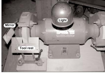
Strong and sturdy tools rests, good lighting, solid mounting and at least one good wheel are minimal requirements for a reliable grinder. The tool rest on the left is after-market rest. A supporting strap was added to the right rest for increased right
