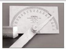
Give a protractor a try. We got a few letters after last issue's grinding article about grinding the correct angle. This metal protractor-available for about \$12-is one inexpensive and reliable solution.
