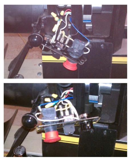
I removed the control panel from the head stock and took a couple pictures with my cell phone so that I would have a reference of which wire went where.
