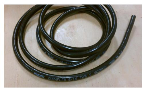
10 feet of trailer wire. They did not have 5 conductor wire, so I got some 6 conductor and didn't use one of the wires.
