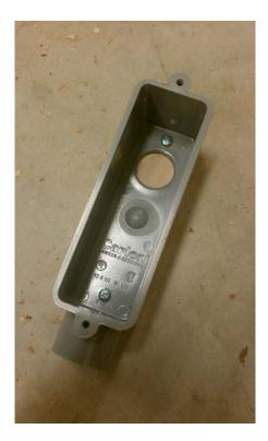
I cut the back outlet thingy off the conduit box at the band saw. Then I cut a piece of scrap wood the size of the conduit box. Epoxied six ½" x 1/8" rare earth magnets into the wood and then screwed the wood to the backside of the conduit box. You need some strong magnets. The on/off switch on the control panel takes quite a bit of force to pull out and if the magnets are not strong enough you will pull the remote box off the lathe trying to turn the lathe on.
