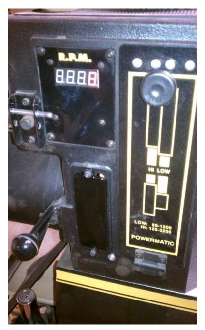
The headstock with the conduit cover in place of the control panel.
