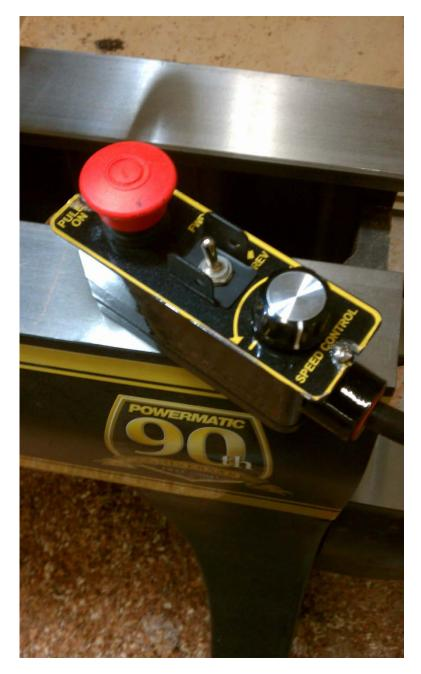
The remote switch. It sticks in the horizontal position better than in the vertical position due to the curved sides of the lathe ways.
