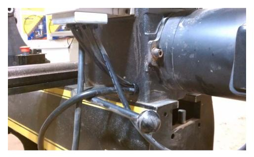
Push the wire through the hole at the back of the head stock. Remove the grommet from the hole first. It's a very tight fit. I couldn't get the grommet back in the hole fully, you might have better luck.
