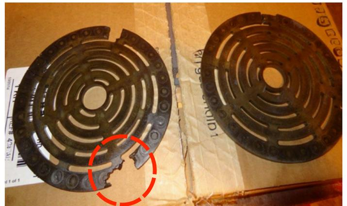
Note: This picture shows a damaged discharge compressor valve following the recommendation of the technician to replace it. Source: [16]
