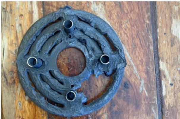
Note: This damage to the compressor discharge valve plate has reduced the compressor capacity by 25%. [16]
