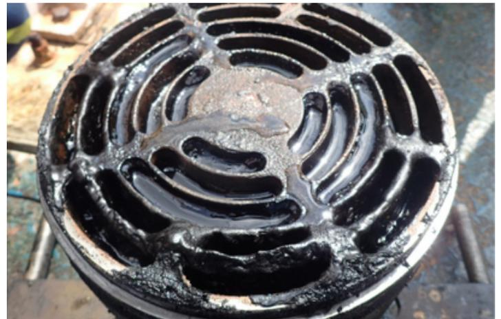
Note: This valve shows excess oil at the point where it is clogged. This was probably due to excess oil from forced lubrication systems. Source: [15]
