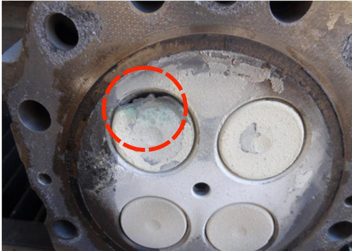
Note: This engine head exhibits an exhaust burnt valve, decreasing its ability to generate power. The issue was identified using ultrasonic diagnostics. Source: [16]
