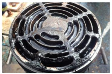
Note: This valve shows excess oil at the point where it is clogged. This was probably due to excess oil from forced lubrication systems. Source: [15]
