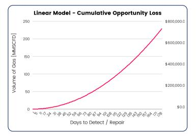
Note: The red curve shows how much money and fuel are lost when a compressor valve starts to leak. It tracks the compressor's capacity dropping from 1% to 25% because of the leak, getting worse over time (this example uses 1380 HP engine & 10 Mmscfd compressor). Cost data is from October 2024. [7] & [8]
