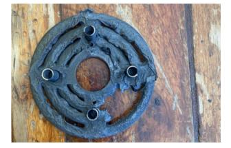
Note: This damage to the compressor discharge value plate has reduced the compressor capacity by 25%. [16]
