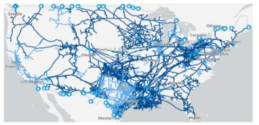
Note: U.S. Energy Information Administration, U.S. Energy Atlas, January 29, 2024. Light-Blue lines are intrastate pipelines, dark-blue lines are interstate pipelines, and + are border crossings. Source:[3]
