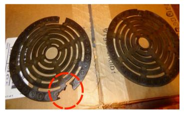
Note: This picture shows a damaged discharge compressor value following the recommendation of the technician to replace it. Source: [16]
