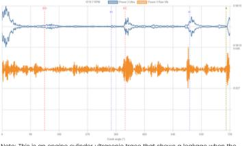
Note: This is an engine cylinder ultrasonic trace that shows a leakage when the piston is on power stroke, indicating a potential issue. Source: [16]
