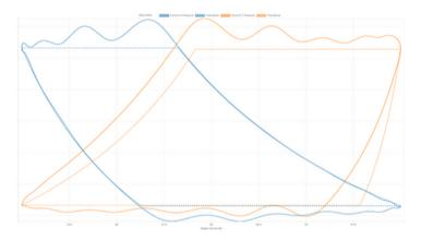
Note: This is a PV plot that exhibit that a compressor discharge valve is leaking. Source: [16]
