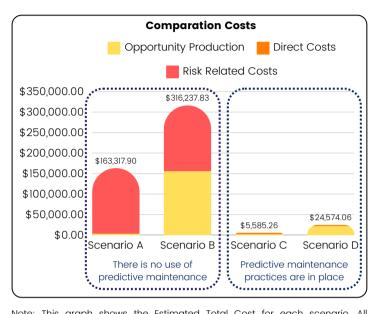
Note: This graph shows the Estimated Total Cost for each scenario. All scenarios use a setup that includes a Cat3500 series and an Ariel Compressor, each capable of handling 10 Mmscfd. Scenarios A and C involve units that are not at fully capacity, while Scenarios B and D use units that are running at full capacity. Source: Author
