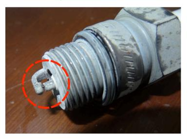
Note: This spark plug has a short circuit between the electrodes, leading to a cylinder misfire, reduced power, and increased torsional vibration. Source: [16]
