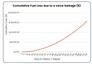
Note: The red curve shows fuel costs during a valve failure, initially rising slowly then accelerating as the failure worsens. It starts with a minor discharge valve leak (reducing compressor capacity by 1%) and worsens to 25% (1380 HP & 10 Mmscfd), assuming no production loss. Cost data is from October 2024. [7] & [8]
