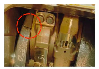
Note: This image shows a crack in the unit's crankshaft, indicating a severe failure that may require anywhere from three days and several months to repair, depending on the availability of resources. Source: [16]
