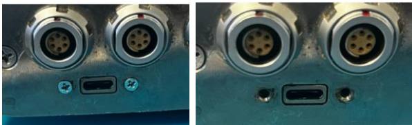
Figure 1. Front USB-C port with screws installed (left) and removed (right).
