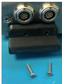
Figure 3. Housing in position with holes aligned; 2-56 screws shown below.
