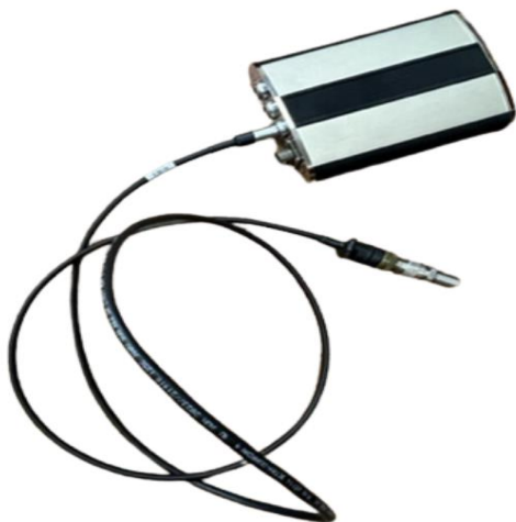
Lenz connected to a Mag Pickup through an Accelerometer Cable, for test purposes only.
