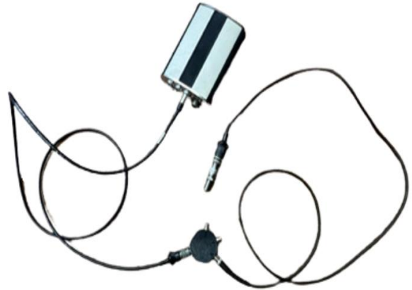
Lenz connected to a Mag Pickup through a XYZ Box, for test purposes only.
