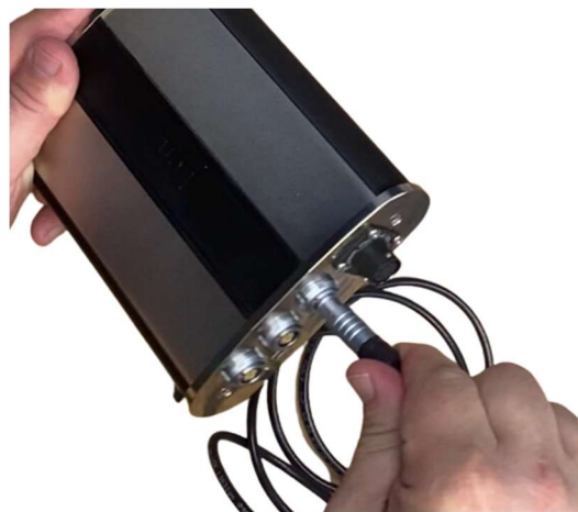
Connecting the Triax Cable to Lenz
