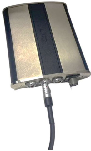
Connecting the Pressure Sensor to the Lenz.
