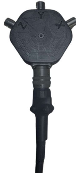
Connecting the Triax to the Cable
