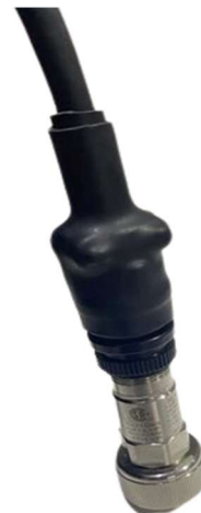
Connecting the Accelerometer to the 2 socket connector
