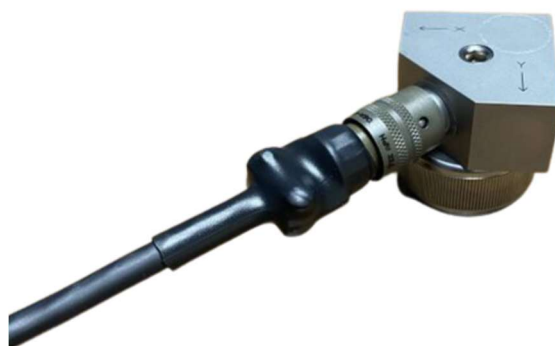
Connecting the Cable to the Triax
