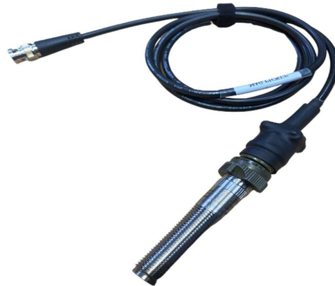
Connecting Magnetic Pick to MagPickup Cable
