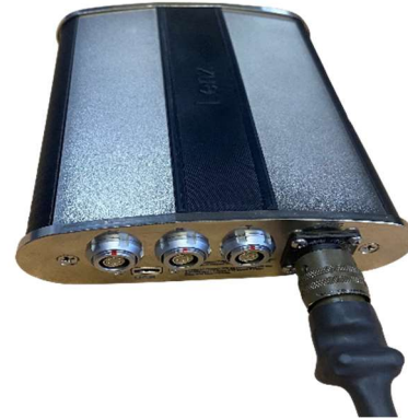
Connecting the Encoder Cable to Lenz.
