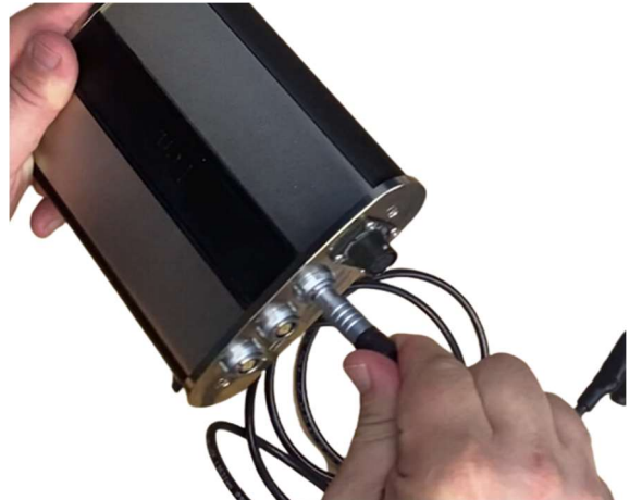
Connecting Secondary Ignition Cable to Lenz.
