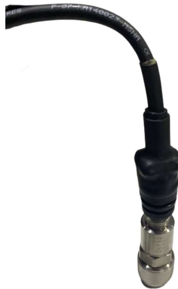
Connecting the Velocity sensor to the 2 socket connector
