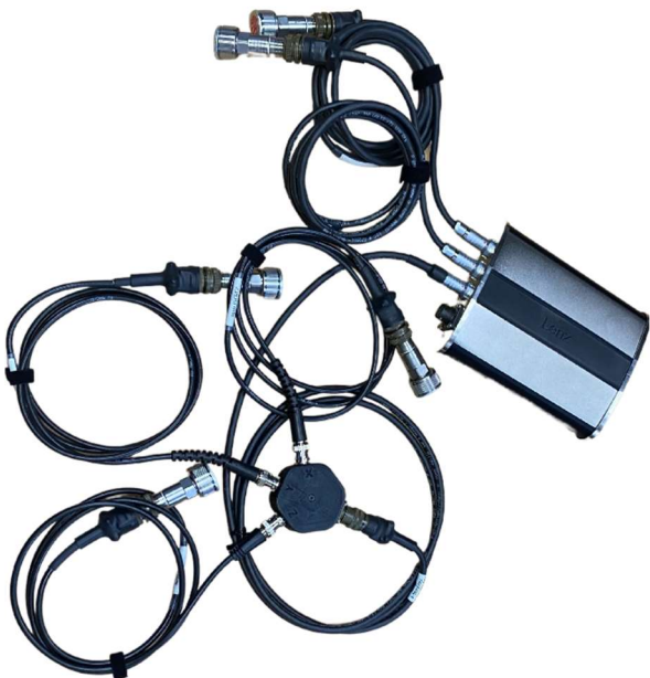
Up to 5 Accelerometers can be connected to Lenz.
