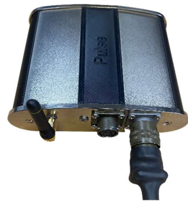
Connecting Encoder Cable to Pulse.
