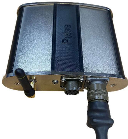
Connecting Encoder Cable to Pulse.
