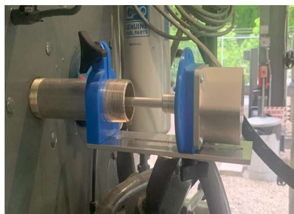
Ariel Kit Mounted on Ariel Crankcase Compressor.
