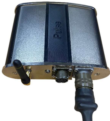
Connecting Encoder Cable to Pulse.
