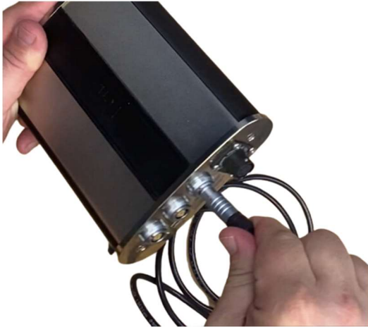
Connecting the Triax cable to Lenz
