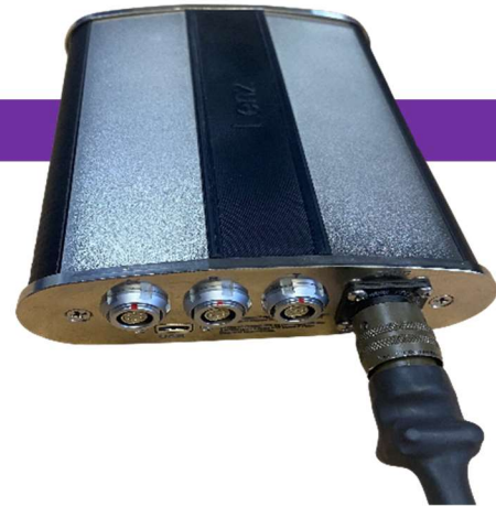
Connecting the Encoder Cable to Lenz.
