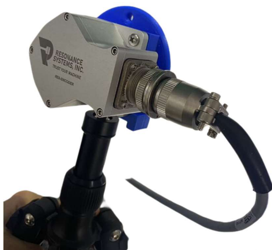
Connecting Encoder Cable to Encoder
