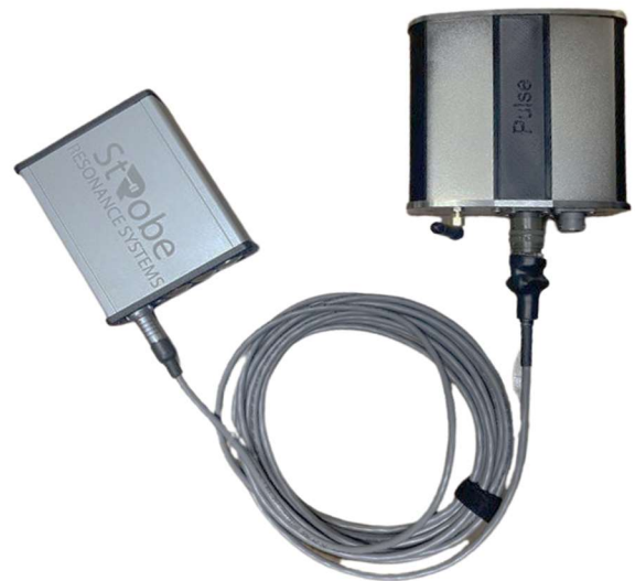
Connecting the Strobe Cable to the Strobe Light
