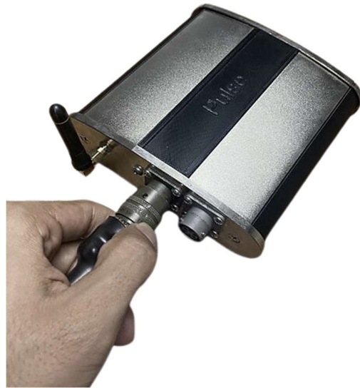
Connecting the Strobe Cable to Pulse.
