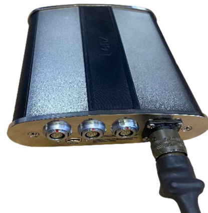
Connecting the Encoder Cable to Lenz.
