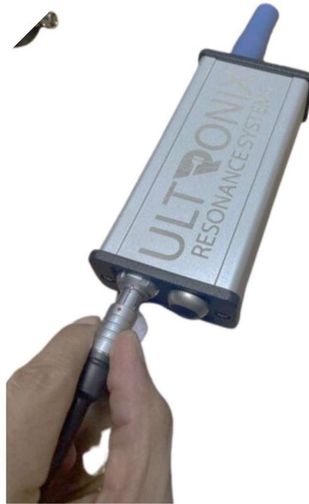
Connecting the cable to the Ultronix.
