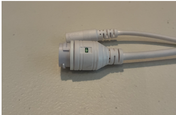
Slip gasket over connector on camera
