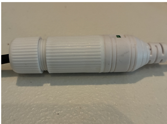
Make the twist connection to the camera
